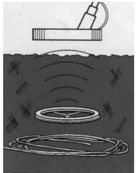
The vertical range of the Mini-Marker is six feet from the locator probe.
